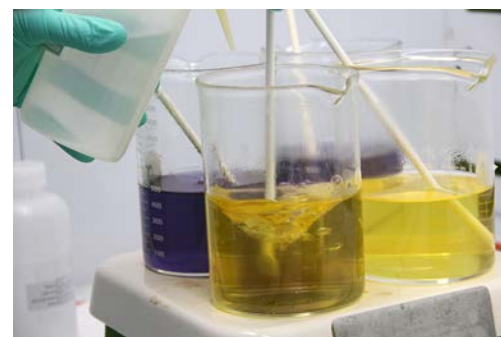
Alpha-emitting radionuclides are co-precipitated with iron hydroxide using a color indicator, bromocresol purple, and a strong base, ammonium hydroxide. Photo: University of Iowa
